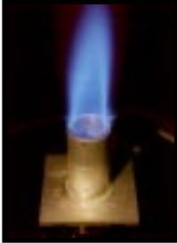
**Technology Benefits:** Patented ring stabilized burner could significantly lower NOX pollution and improve energy efficiency of gas appliances.
