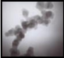
**Soot Micrograph:** Microgravity combustion research has practical significance to a variety of problems in everyday life, such as combustion-generated pollutants.
